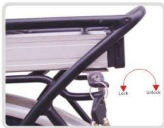
fig.5 (lock/unlock the battery pack to/from carrier)
