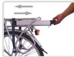
fig.6 (remove/install the battery pack from/to carrier)
